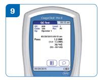
The sample will be analysed and the result and acceptable range displayed on the screen.
