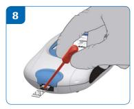
Once the 3 minute countdown starts, apply the solution to the test strip using the pipette.
