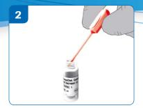
Ensure no liquid is in the end of pipette and carefully cut end off and empty all contents into glass vial, ensuring not to touch the powder. Exercise normal precautions when handling laboratory reagents.
