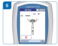
Insert test strip when prompted and test strip code chip (if prompted).
