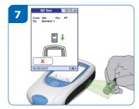
If 'New' option selected, insert QC code chip when prompted or select 'Scan' and scan the side of the QC bottle using the barcode.
