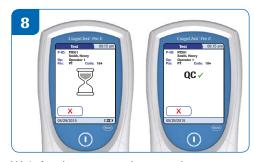
Wait for the meter to beep and start to analyse the sample then remove the finger. The meter will automatically test the on-board QC.
