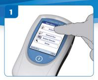
If the function Operator ID is active then log in as the operator and touch 'Patient Test'. If the function Operator ID is inactive, from the Main Menu, touch 'Patient Test'.
