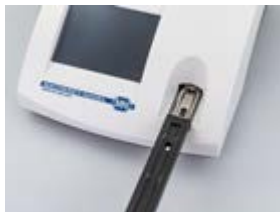
Pic. 20: Reinsertion of the test strip holder
